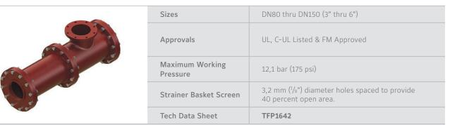
The Model B-1 Pipe Line Strainers are designed for installation in the water supply connection to automatic sprinkler, water spray deluge, foam-water deluge, or standpipe fire protection systems.
