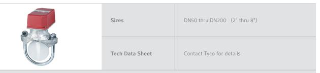
Vane type waterflow switch for use on wet sprinkler systems Actuated with a minimum flow of 10 gallons per minute Retard delay is an adjustable feature that can be set from 0 to 90 seconds Flow condition must exist for the period of time necessary to overcome the selected delay period
