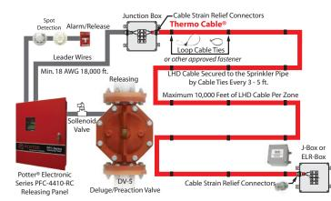
Linear Heat Detection Cable allows a Quell designed fire sprinkler system to be more efficient by quickly recognizing the fire, and conveying the information back to the fire alarm panel.
