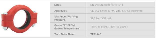
The GRINNELL 707 Flexible Coupling provides a dependable method of joining pipe and is suitable for use in a variety of applications Capable of pressures up to 34,5 bar (500 psi) depending on pipe size and wall thickness Also available with tri-seal Grade "E" EPDM gasket for dry pipe fire protection systems, vacuum systems, and freezer applications
