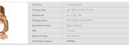
Early Suppression, Fast Response (ESFR) a 3mm bulb type Primarily designed for use in ceiling only sprinkler systems Use of this sprinkler is especially advantageous as a means of eliminating the use of in-rack sprinklers when protecting rack storage arrangements Available in two temperature ratings and Listed or Approved accordingly; 155°F (68°C) is UL and C-UL Listed and FM Approval; and 200°F (93°C) is UL and C-UL Listing only.
