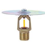
3 mm bulb Intermediate level with shield Factory assembled unit having an integral water shield Used where sprinkler guards are not required
